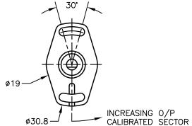
SHAFT FLAT ALIGNED WITH REFERENCE MARK IN BASE AT MID TRAVEL ±5"
